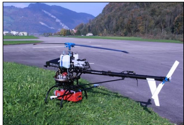
Figure 1: The Scout B1-100 UAV with the integrated laser scanning payload.
