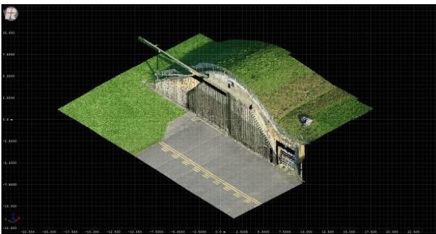
Figure 6: Section of the LiDAR point cloud representing the airplane hangar in Fig. 5 after post-processing.
