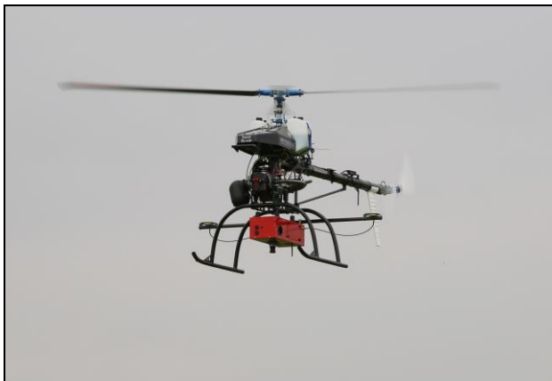
Figure 4: The Scout B1-100 UAV helicopter equipped with the hyperspectral camera during data recording.
